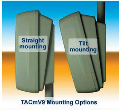
Decide if you want straight (left picture) or tilt mounting. The wall mount conduit entry points are at the bottom for straight mount and at the top for tilt (approx 15 degrees) mounting.
