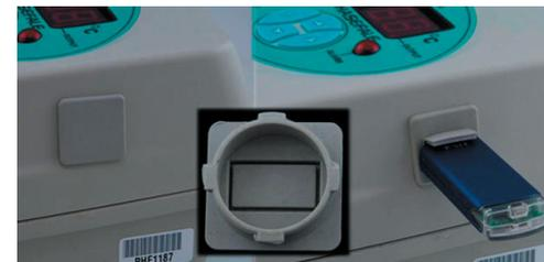
The USB plug provided can be left as is when logging is not required and no memory stick fitted. When logging is employed, cut 3 sides of the plug to allow a flap which raises for the memory stick as shown in the photo below.
